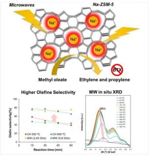
Fig. 1. Design and performance of the proposed microwave-heatable catalyst. Researchers from Kyushu University used microwaves to heat up a sodium-substituted zeolite catalyst, Na-ZSM-5, so that it could more efficiently convert biomass to useful industrial precursor chemicals. without harmful side effects. (Kyushu University/Shuntaro Tsubaki)
